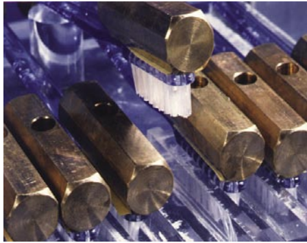
Fig 6: Each toothbrush carries a weight of 100g
