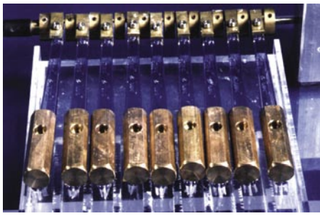
Fig 5: Brushing Machine: nine brushes are simultaneously brought into motion
